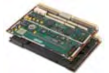
EP2A 6U VME, air or conduction cooling, dual PMC sites
